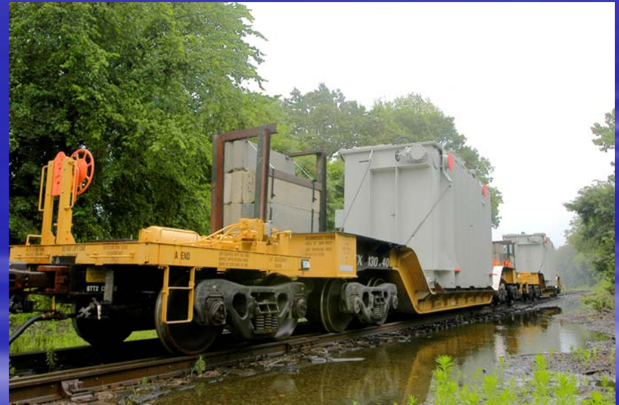
Shunt reactors transported by rail
