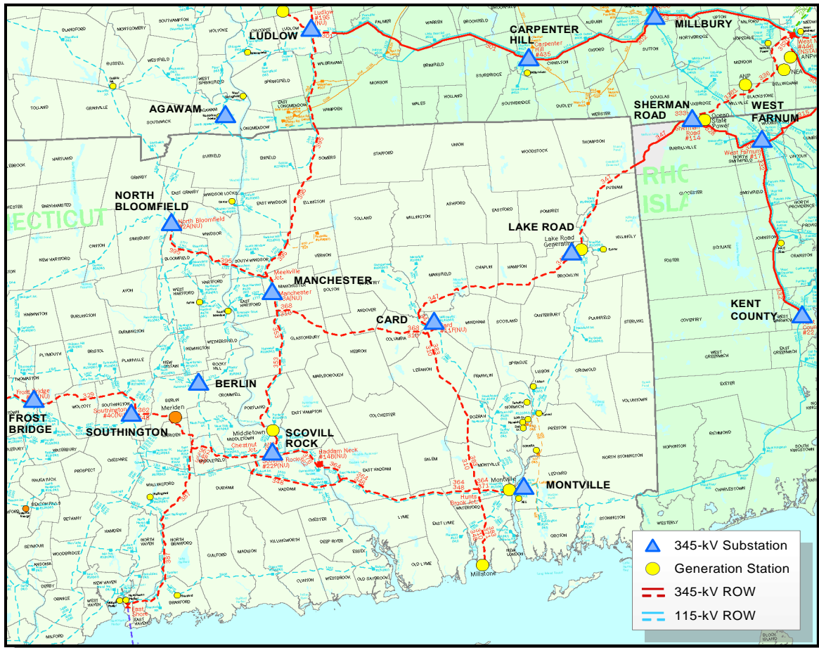
Figure 1-1: Key substations in southern New England.
