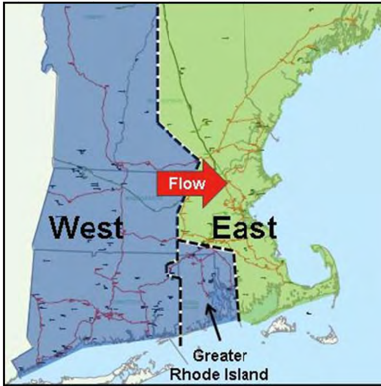
Figure 2-7: East – West Interface and Greater Rhode Island Corridor Limit Flows From the West and Greater Rhode Island to the East
